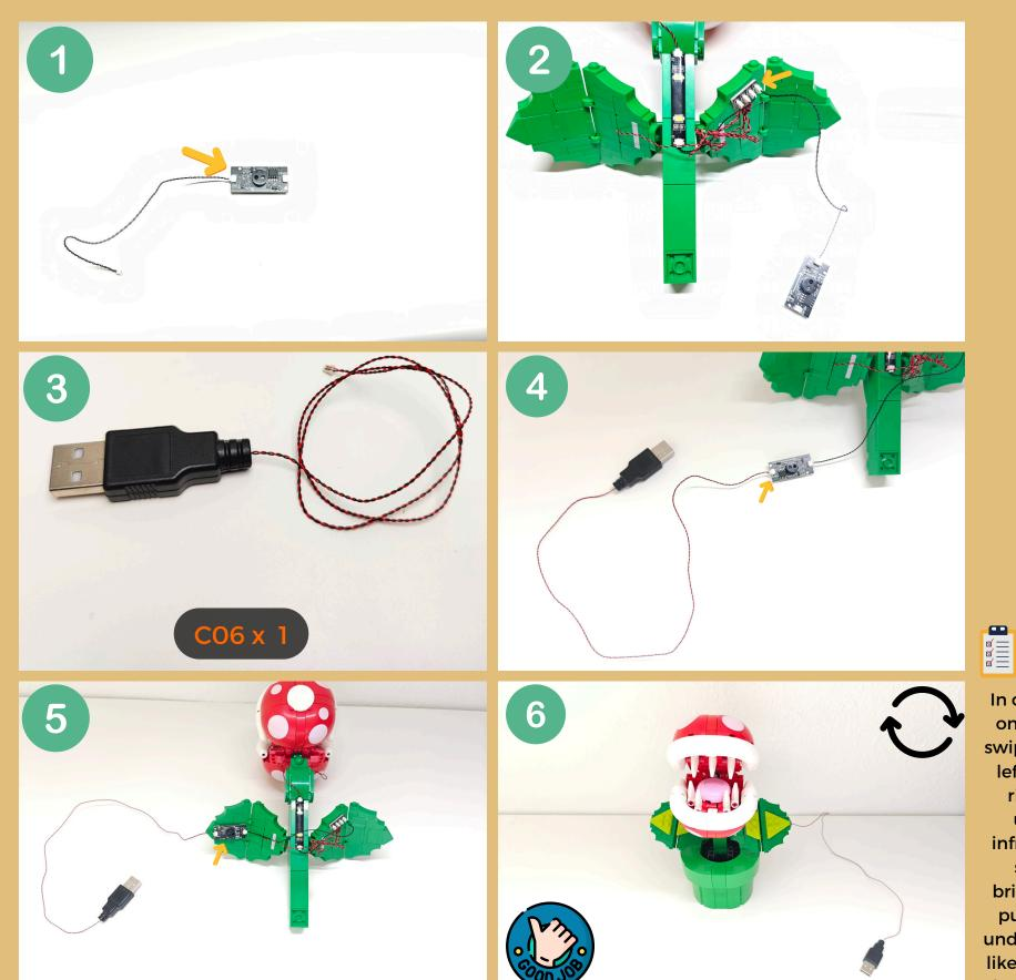
In order to turn on the model; swipe your hand left to right or right to left under the infrared sensor swith. For brightness just put you hand under the sensor like a automatic hand sanitizer.
